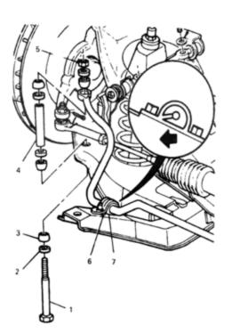
There are two ways to eliminate the chirp: (1) replace the sway bar bushings - or (2) grease the bushings on your car. Either of these two options require roughly the same amount of labor to complete, so I would strongly recommend replacing the bushings, if you are experiencing this "chirp" on your 1988 model Fiero.
