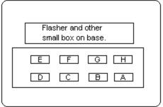
The Chime Socket looking at the base from under the dash: This side is most distant from flasher & fuse on the same base.
